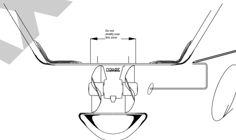
Fit the tunnel and mark the areas to be fiber-glassed. Sand these areas inside and out.
